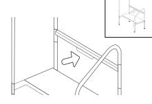
Peel two-sided tape off back of light (G) and attach to light bracket on part C with light & sensor facing out. See other side for details.
