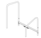
Insert A & B into holes of part C (Part A towards head of bed) (Part C with light bracket underneath cross bar)
