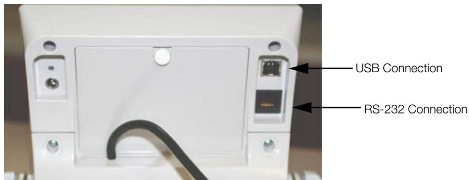
Figure 5-1. USB Connection Port and RS-232 Connection Port
