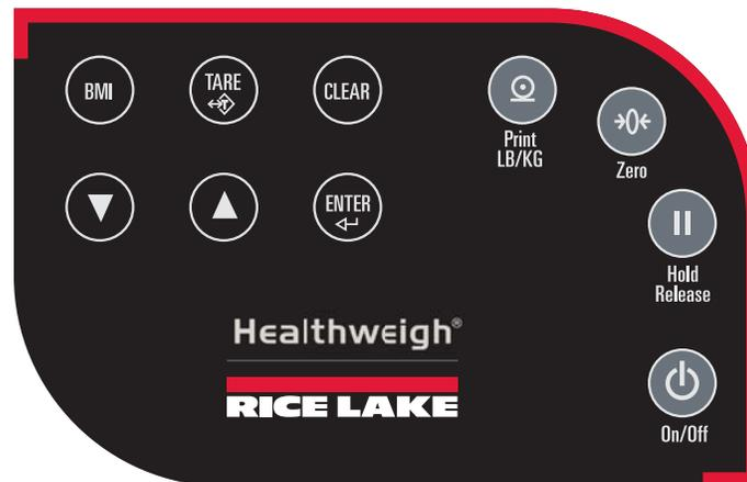
Figure 4-1. Front Panel Display Keys
