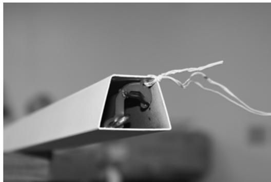
*Figure 2-2. Remove Cable Tie From Lever*
