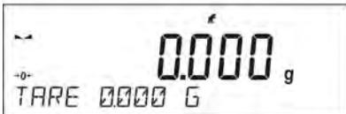
Place the container in which the measurement is to be carried out on the weighing pan and when the indication is stable tare its mass.
