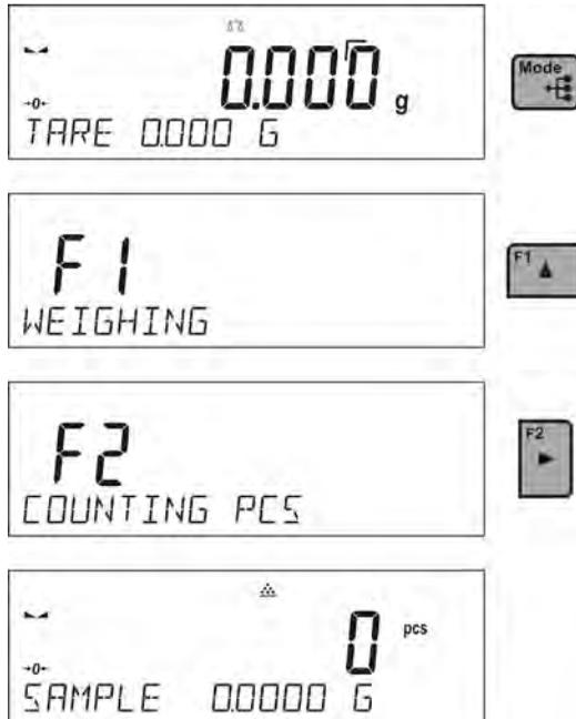
When the function is initiated for the first time, the standard mass equals 0.0000g. If the sample mass is determined and has been used in the mode <COUNTING PIECES> then the software accepts the mass of recently used standard as the standard mass.
