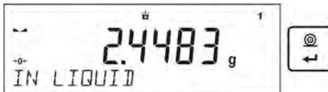
12. On the second measurement result approval, the program will automatically calculate the tested solid object density and it will be indicated on a balance display. At the same time, the measuring report will be sent to a selected printer port
