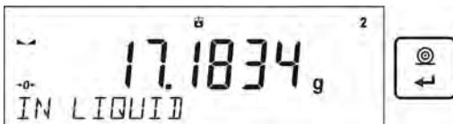
10. On the second measurement result approval, the program will automatically calculate density of the tested liquid which will be indicated on the display. The measuring report will be sent to a selected printer port
