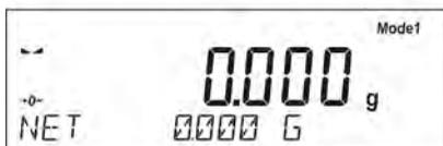
Once you select the mode, the function is activated and the information about the net mass appears in the bottom line (only if a different mass has not been selected by a user).
