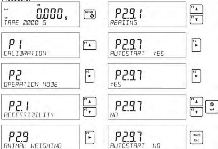
After altering the setting, return to the main window by pressing **Units Esc** button repeatedly.
