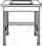
It is a very stable basis which eliminates all kinds of vibrations and ground shakes. The inner part of the table holds a marble plate, which is a foundation for balance positioning.
