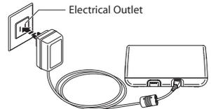
**NOTE:** AC adapter can be worked at 100 - 240V ~ 350mA, 50/60 Hz.
