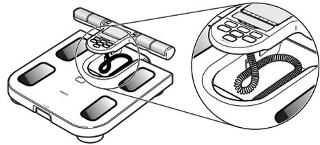
3. Place the Display Unit into the Display Unit Holder.
