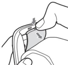
2. Insert 2 “AAA” alkaline batteries as indicated in the battery compartment.
