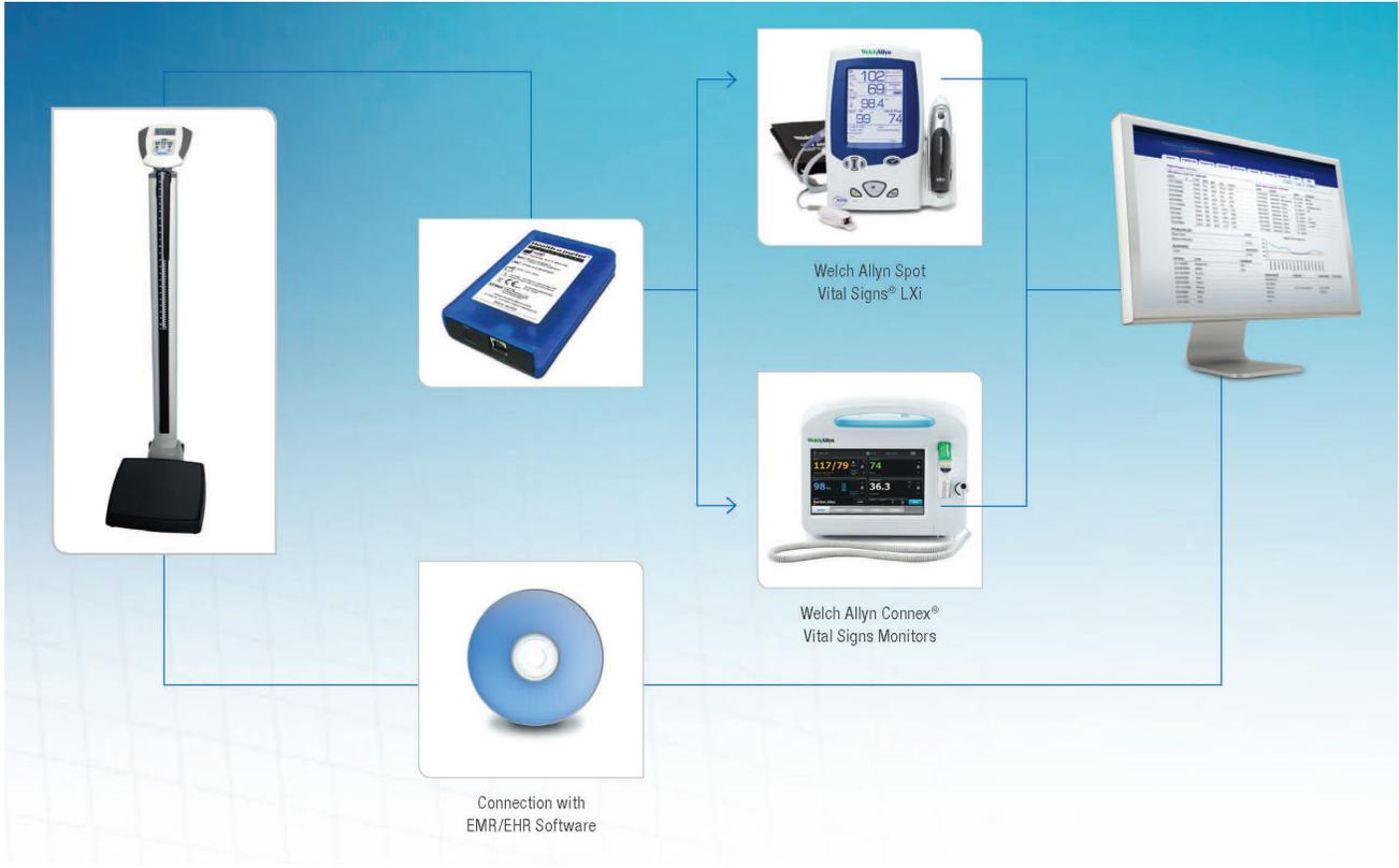
The **L-HOMWA-1** Connectivity Kit is intended to be used with the Welch Allyn Spot LXi Monitor. It is designed to be utilized in environments where the intended use is monitoring weight, height and BMI of patients in hospitals, and hospital-type facilities that utilize the Welch Allyn patient monitoring systems.
