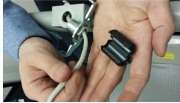
5. Remove the silver display mount and bolt from the load cell cable. Separate the bolt from the mount and retain the bolt for use in step 7.
