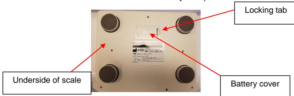
2. Replace or install a new 9V battery. Health o meter<sup>®</sup> Professional recommends using an alkaline or lithium battery, rated for 130°F (54°C) operation. Do not use zinc-carbon batteries. Reattach the battery compartment door.
