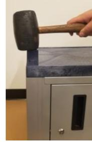
4. Carefully turn over the assembled cabinet. Insert the stems of the two casters with locks into the holes on the front of the cabinet with the door. Push in casters until fully seated. Gently tap with rubber mallet if needed. Lock the two locking casters to aid in further assembly.
