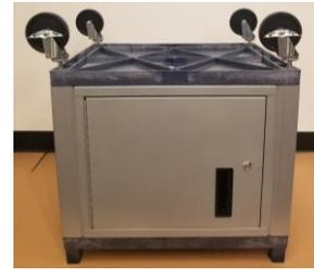
6. Turn the cart over, upright on all four casters and shelf mounting posts facing up. Ensure cart is level with all four casters fully seated. If needed, tap down on the top surface to completely seat the casters.
