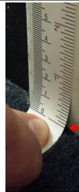
10. To verify that the measuring tape is at the accurate height in the height rod channel, place a tape measure flush against the floor and against the side of the height rod channel. Check that the height measurement on the height rod matches the height shown on the tape measure. To adjust, slide the height rod measuring tape until it matches the reference height shown on the tape measure.
