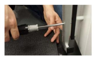
7. Once all 3 screws are inserted, fully tighten the screws starting with the bottom. Ensure that the screw extends completely through the mounting bracket as shown. Assembly is now complete. See the next page for usage instructions.
