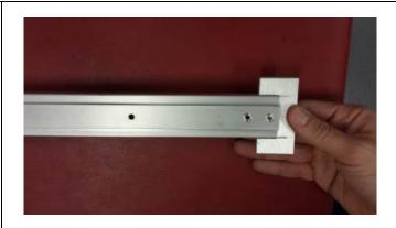
2. Use a rubber mallet to completely insert the footpiece onto the height rod so that the ends are flush.
