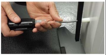
6. Obtain the height rod from the carton and extend it fully. Insert one of the #8 screws into the bottom hole on the height rod then into the bottom hole on the black mounting bracket that is attached to the pillar. Do NOT fully tighten the screw at this point. Repeat the process with the two remaining #8 screws and insert them into the top and middle holes in the height rod then into the mounting bracket.
