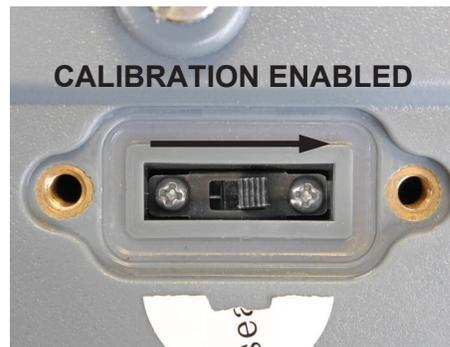
3. Move the calibration switch to the right as shown in the right image above.
