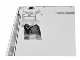
4. Install the 9VDC battery.
