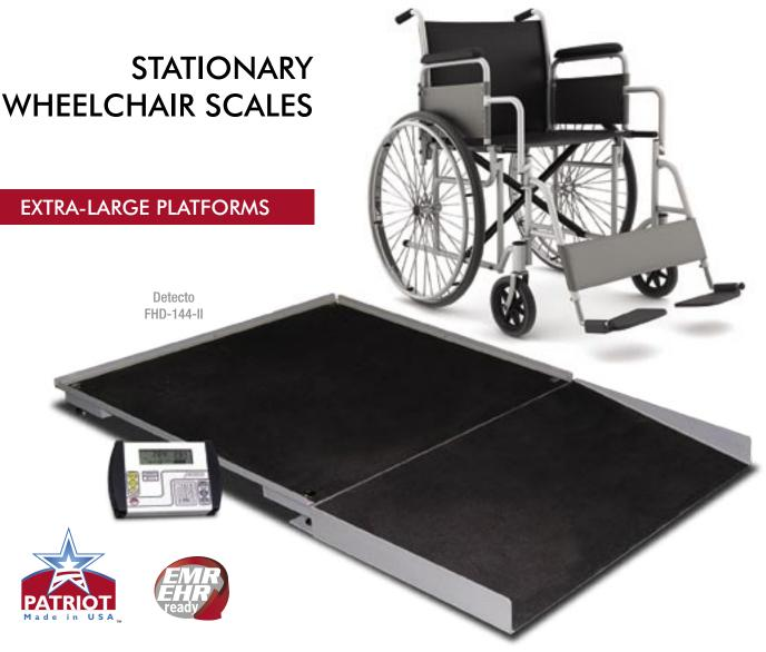
The large slip-resistant platform of Detecto's FHD scales accomodate walk-on patients, wheelchairs, straight-legged chairs, or walkers. These scales feature a high 1,000 lb / 450 kg capacity with your choice of 36 in / 91 cm or 48 in / 122 cm square platforms. The weight indicator provides EMR/EHR-ready output via serial, USB, or optional Ethernet ports. This scale can only be used for top of floor installations. Please consult factory for pit type installations.
