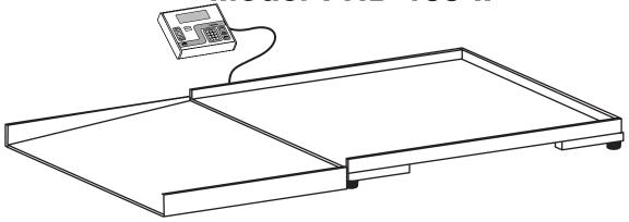
The battery operated Model FHD-133-II Geri-chair scale has a nonskid platform and ramp. The large platform accommodates walk-on patients, wheelchairs, or straight-legged chairs. This large capacity scale can be mounted flush with the floor if desired. The remote digital weight display includes .7 high LCD readout with keypad tare and is suitable for desk or wall mounting.
