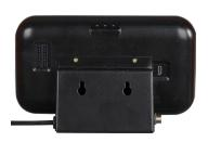
The indicator comes with (1) RS232 serial port and (1) micro USB-B port, plus Wi-Fi/Bluetooth is available
