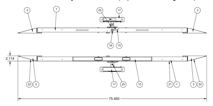
8500 Final Assembly – 0065-0809-0A Section A-A, Section B-B, and Section C-C Views
