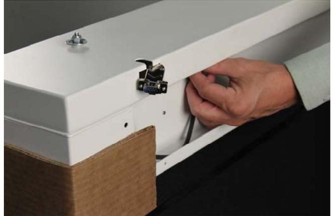
3. Feed the load cell cable through the large cut-out in the back of the scale frame.
