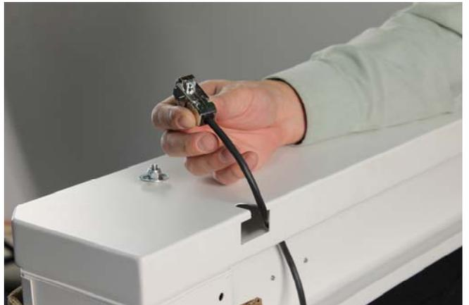
4. Continue feeding the load cell cable through the scale frame and up through the notch in the top of the scale frame.
