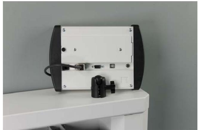
3. To install the indicator, slightly loosen the adjustment knob to allow the two parts of the socket to open enough to insert the rubber ball and place the rubber ball on the back of the indicator into the swivel ball socket mount. Tighten the adjustment knob slightly to secure the indicator for the next step.
