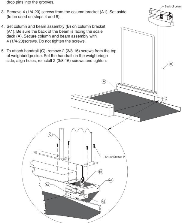
6. If available, place the scale on a table or workbench, otherwise place the scale on floor. In either case, **DO NOT** tilt or place scale on it's side. Next, push bottom of the hanger (B1) back towards the scale weighbridge (A), lift long lever and the nose iron (A2) up, slide the hanger (B1) under the nose iron pivot (A3). After the hanger is attached, tighten the 4 (1/4-20) screws. The scale assembly is now complete.
