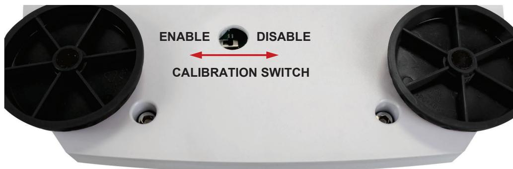
1. Turn the scale over so that the feet are facing up, locate the calibration seal between the front feet, and break (cut open) the calibration seal.
