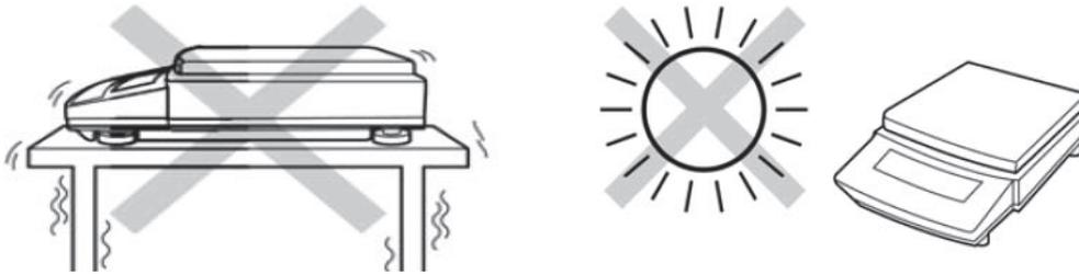
Do not place the scale in locations with excessive temperatures and humidity. For example, directly in front of a heating or cooling vent, a fan, window, or any location with a moving air source. Such a location will subject it to sudden temperature changes, which may result in unstable weight readings.
