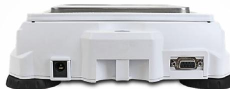
RS232 serial port located on the back of the scale that may be used to send weight and associated data to a printer or other RS232 device. The port can be configured to send data continuously, send when a stable weight is obtained, or when the **PRINT** key is pressed.
