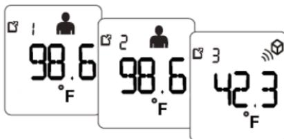
**Note:** The Human or Object symbols will be displayed to indicate the measurement mode that was in use for the displayed reading in memory.
