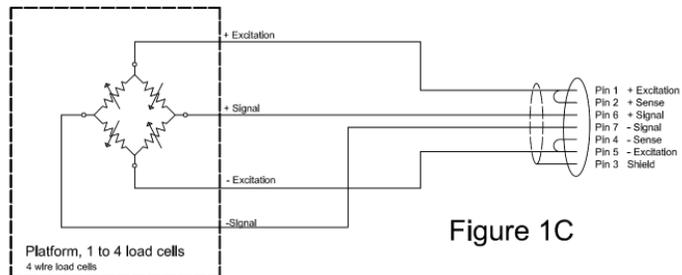
Figure 1A shows the connections to a 6 wire load cell. Figure 1B and 1C show 2 different ways to attach a 4 wire load cell, 1B uses a 6 conductor cable to go from the indicator to the platform or load cell where it connects to the 4 wires from the load cells.
