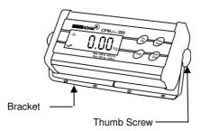
To adjust the angle of the indicator, use the two thumb screws on the side of the bracket that connects the indicator.
