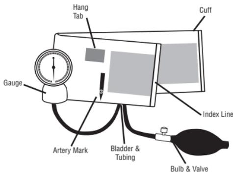
Most models come preassembled and ready for use. If assembly is required, attach gauge and bulb and valve assemblies to the tubes as shown in illustration. To facilitate, use alcohol or soapy water.
