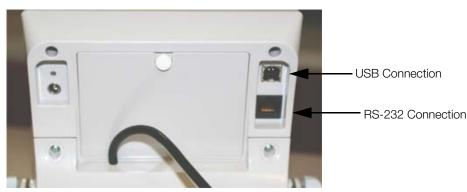
Figure 5-1. USB Connection Port and RS-232 Connection Port
