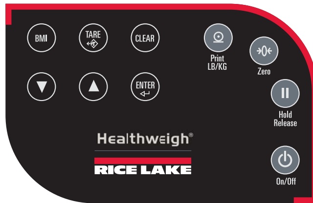
Figure 4-1. Rice Lake Digital Floor Level Scale Front Panel Display Keys
