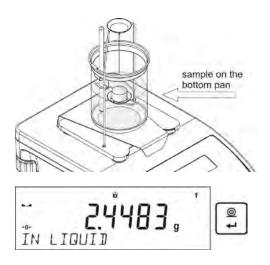
12. On te second measurement result approval, the program will automatically calculate the tested solid object density and it will be indicated on a balance display. At the same time, the measuring report will be sent to a selected printer port
