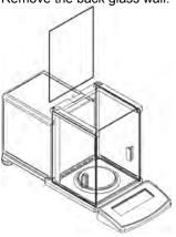
3. Remove the side glass walls. The side glass walls are not replaceable, so it is important to remember which one is left and right, and after cleaning install them back properly in the draft shield.
