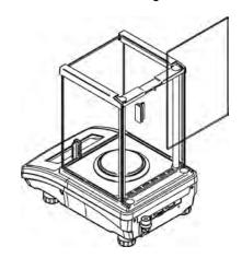
3. Remove the side glass walls. The side glass walls are not replaceable, so it is important to remember which one is left and right, and after cleaning install them back properly in the draft shield.
