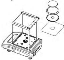
Thus prepared draft shield and glass walls can be properly cleaned. All the operations should be done carefully. Pay special CAUTION to the place where the weighing pan was installed: dirt and other small elements might enter the balance construction through this openiing, which might negatively influence the balance parametres.
