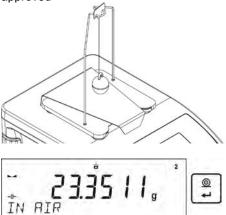
9. Next, take the sinker out of the hook and put the tested sample with liquid on the beaker's basis (the beaker cannot touch the hook). Delicately hang the sinker on the hook (the sinker must be totally emerged in the tested liquid) – a mass sample determination in liquid – and after the indication stabilization approve the result.
