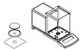
Thus prepared draft shield and glass walls can be properly cleaned. All the operations should be done carefully. Pay special CAUTION to the place where the weighing pan was installed: dirt and other small elements might enter the balance construction through this openiing, which might negatively influence the balance parametres.
