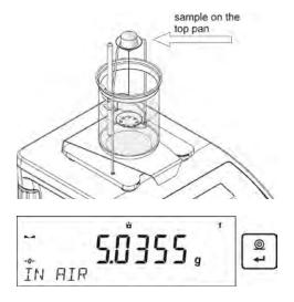
11. Next, a mass sample should be placed on the bottom pan of the kit (mass determination in the liquid), and after the indication stabilization, approve the result
