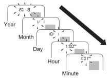
**3.** Press the [START/STOP] button to store the setting. It automatically turns off after 3 seconds.
