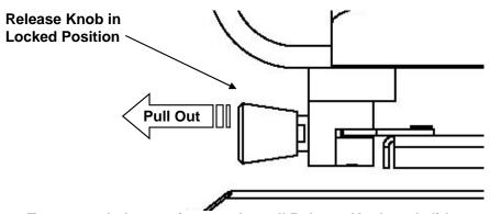
To remove baby tray from scale, pull Release Knob and slide tray off weighbridge.
