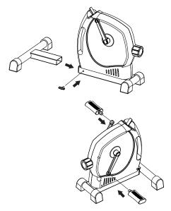
**Step 1** Insert the Front support tube into the body assembly and adjust it to the desired position. Then attach the locking knob and tighten it.
