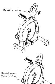
**Step 3** Plug the monitor wire to the monitor and slide monitor completely onto mounting tab.
