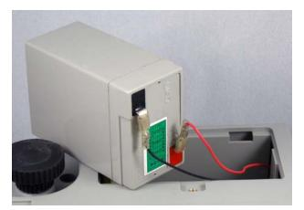
Connect the red wire to the red battery terminal and the black wire to the black battery terminal.
