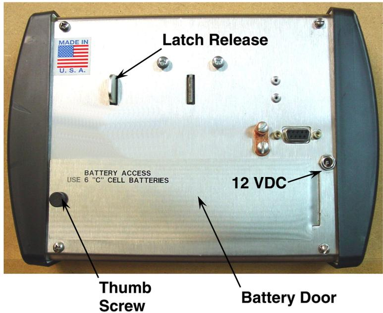
5. If installing new batteries, proceed to step 6. If replacing the batteries, remove all 6 batteries from the battery holder and then proceed to step 6.
